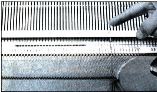
7. Hook the another yarn into the HOOK of these needles, and make a stitch as shown in the figure.
